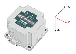
IMU560 use NED coordinate, right hand coordinate, axis direction above. By the rotation direction Z-Y-X, when X forward direction point to the front of carrier, then the angle rotating Z axis is yaw, Y axis pitch, X axis roll.
